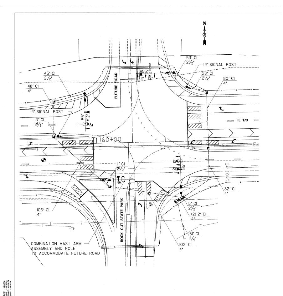
I. THE MOUNTING HEIHT FOR THE LUMINARIES SHALL BE 35'0" TENON MOUNTED WITH AN 8'HORIZONTAL ARM
