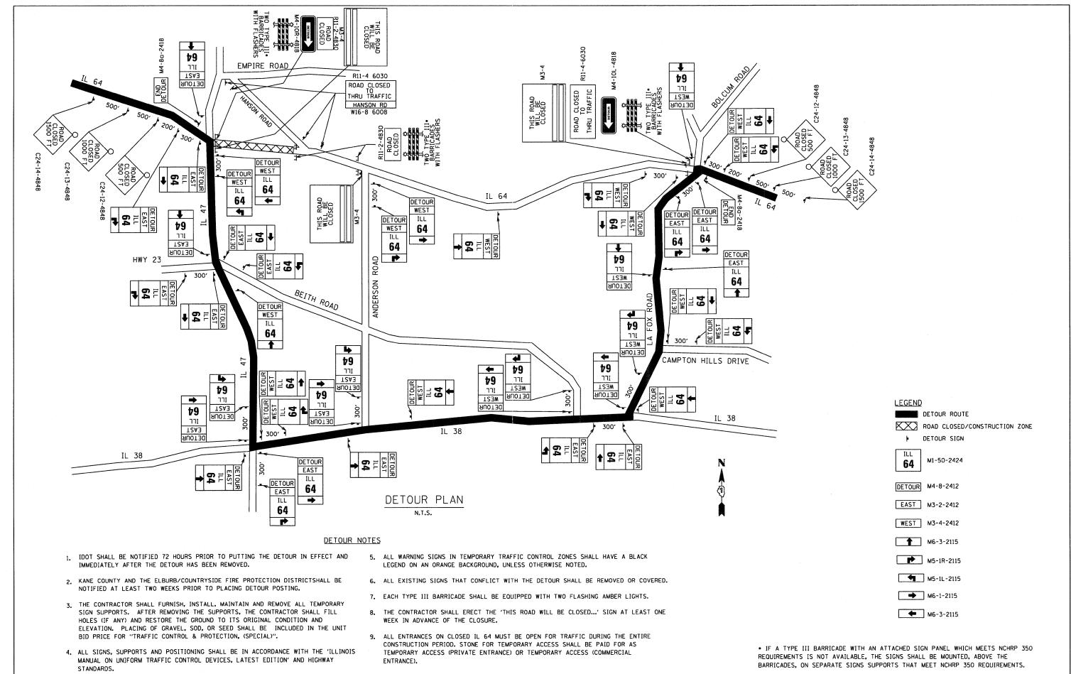
DESIGNED - AR REVISED FILE NAME = USER NAME = \_USER\_ SECTION COUNTY SHEETS NO. IL 64 AT IL 47 INTERSECTION IMPROVEMENTS STATE OF ILLINOIS REVISED \$FILEL\$ DRAWN KANE STAGE 1 DETOUR PLAN - EAST LEG IL 64 PLOT SCALE = 50.0001 ' / IN. CHECKED -RS REVISED **DEPARTMENT OF TRANSPORTATION** CONTRACT NO. 62278 REVISED SCALE: SHEET NO. 1 OF 1 SHEETS STA. PLOT DATE = 9/1/2011 DATE
