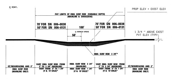
\*MILL TO A DEPTH OF 2 1/2" UNDER SN 006-0131. THE PROPOSED TOTAL OVERLAY TOTAL RESURFACING THICKNESS SHALL BE 2 1/2" UNDER SN 006-0131. PLACE TWO LIFTS OF SURFACE COURSE WITH EACH LIFT 1 1/4"
