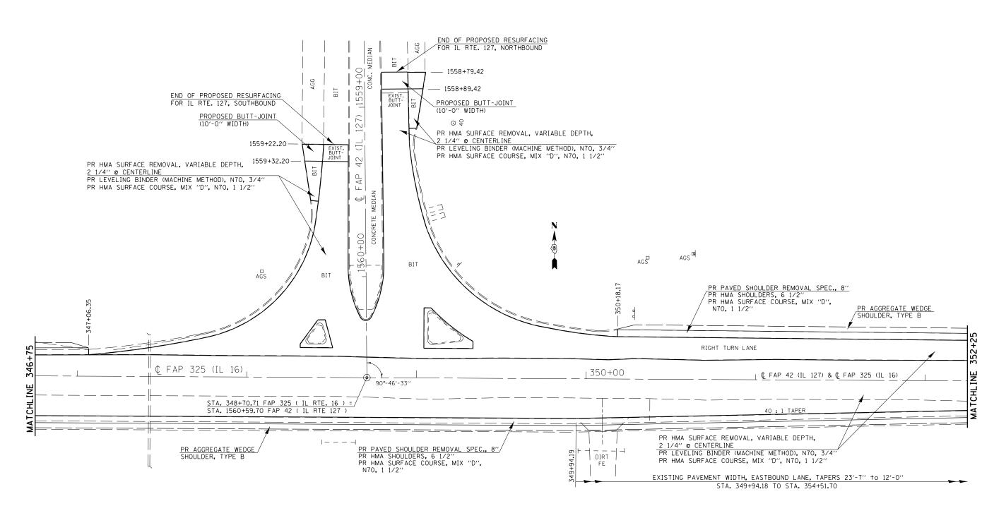
THE PROPOSED PAVEMENT STRIPING IS NOT SHOWN ON THIS PLAN SHEET. SEE THE PROPOSED PAVEMENT MARKING SHEETS AND SCHEDULES FOR MARKING LOCATIONS. WIDTH OF PROPOSED SHOULDER REMOVAL AND HMA SHOULDERS IS 4' UNLESS OTHERWIZE STATED WITHIN THESE PLANS. WIDTH OF PROPOSED AGGREGATE SHOULDER WEDGE, TYPE B IS 3'-0".
