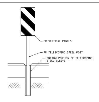
NOTE: FOR INSTALLATION OF VERTICAL PANELS IN AREAS OF CROSSOVER PAVEMENT, 3" Ø HOLES WILL BE CORED THROUGH PAVEMENT FOR PLACEMENT. TELESCOPING STEEL POLES WILL BE PLACED I" BELOW SURFACE AS SHOWN, AND WORK SHALL BE DONE TO THE SATISFACTION OF THE ENGINEER, WHEN OPENING CROSSOVER, PANELS WILL BE REMOVED AND HOLES WILL BE LEFT IN PLACE. COST OF PANELS, POSTS, SLEEVES, TYPE III BARRICADES, SIGNS, AND CORING SHALL BE INCLUDED IN MEDIAN CLOSURE.
