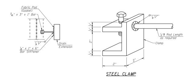
Notes: Pop rivet the 'g" x 1" bar to Drain Extension. Weld or securely attach rod to both the clamp and bar stiffener. Use <sup>3</sup><sub>16</sub>" stainless steel pop rivets of sufficient length. Clamp shown in approximate dimensions. Similar commercially available may be substituted.
