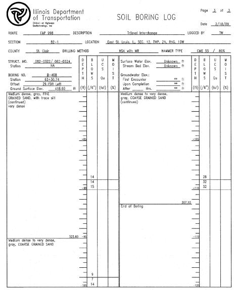
The Unconfined Compressive Strength (UCS) Failure Mode is indicated by (B-Bulge, S-Shear, P-Penetrometer). The SPT (N value) is the sum of the last two blow values in each sampling zone (AASHTO 1206).
