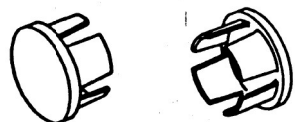
CAST END CAP DRIVE FIT TYPE 3 - Required Incidental to item "Aluminum Handrail"
