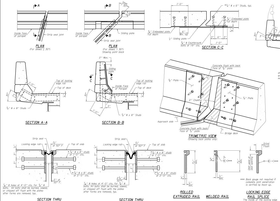
SECTION THRU ROLLED RAIL JOINT
