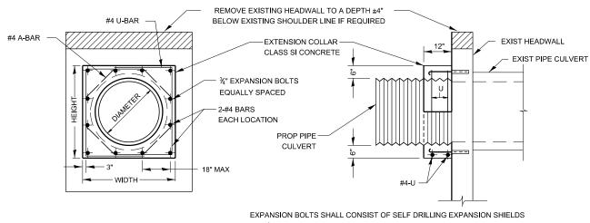
AND  $\frac{3}{4}$ " DIA HOOKED BOLTS. HOOKED BOLTS SHALL EXTEND A MINIMUM OF 9" INTO NEW CONCRETE. MINIMUM CERTIFIED PROOF LOAD = 4,080 LBS
