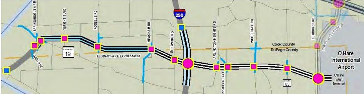
The other major roadway component of the build alternatives is the O’Hare West Bypass extending from I-90 to I-294 about 6.2 miles along the west side of O’Hare Airport (see figure to the right). For Alternative 203, the bypass would be a freeway for the entire length. However, for Alternative 402, only the southern portion of the bypass would be a freeway, and the northern portion would be an arterial improvement along York Road/Elmhurst Road.
