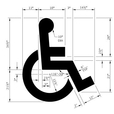
TYPICAL DETAIL FOR PAINTING HANDICAP MARKINGS
