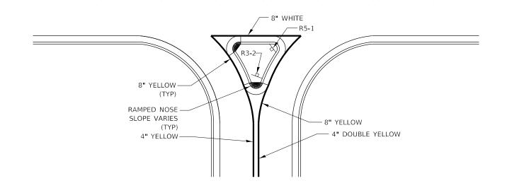
RIGHT IN RIGHT OUT ACCESS PAVEMENT MARKING
