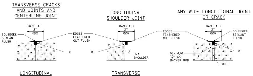
\* HOT ASPHALT CRACK SEALANT APPROX.  $\frac{3}{4}$ " ×  $\frac{3}{4}$ " × LENGTH OF CRACK (19 mm × 19 mm × LENGTH OF CRACK)
