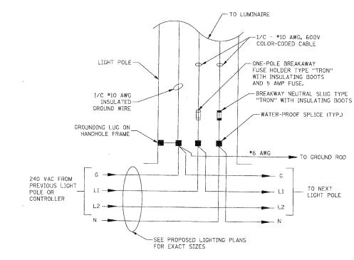
LIGHT POLE HANDHOLE WIRING DETAIL
