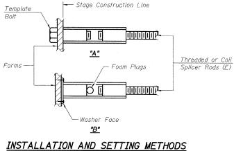
"A": Set bar splicer assembly by means of a template bolt. "B" : Set bar splicer assembly by nailing to wood forms or cementing to steel forms. (E): Indicates epoxy coating.
