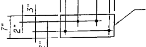
FIXED BEARING R AND NOMINAL SHIM At Relief Joints of Double Girder Spans Stringer Lines 1 & 8 only
