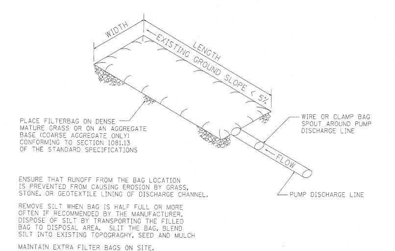
FIGURE S1. SEDIMENT FILTER BAG
