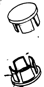
CAST END CAP DRIVE FIT TYPE Q Required Governor to ASTM A-533 Incidental to Item "Metal Handrail"
