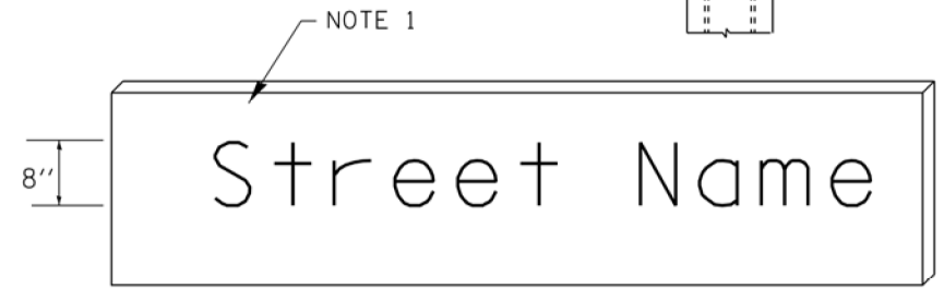
LED ILLUMINATED SIGN PANEL
