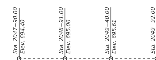
EXISTING EB US 136 PROFILE GRADE (Along median edge of pavement; from survey)
