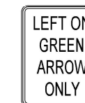
R10-5 30" X 36" D FURNISH & INSTALL FOUR (4) EACH SIGN DETAIL OF SIGN PANEL - TYPE 1 (NOT TO SCALE)
