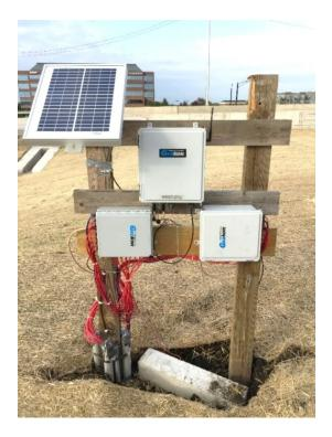
The Contractor shall assist the researchers in the installation of a lightning protection system (rods inserted/embedded in the ground, supplied by researchers) to the data collection locations. The data collection location is where the data acquisition equipment is installed. See photo below.
