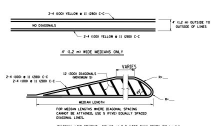
DIAGONAL LINE SPACING: 50' (15 m) C-C (LESS THAN 30MPH (50 km/h))
