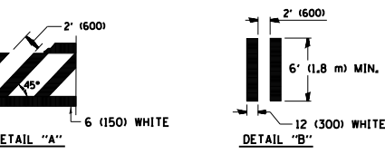
TYPICAL CROSSWALK MARKING
