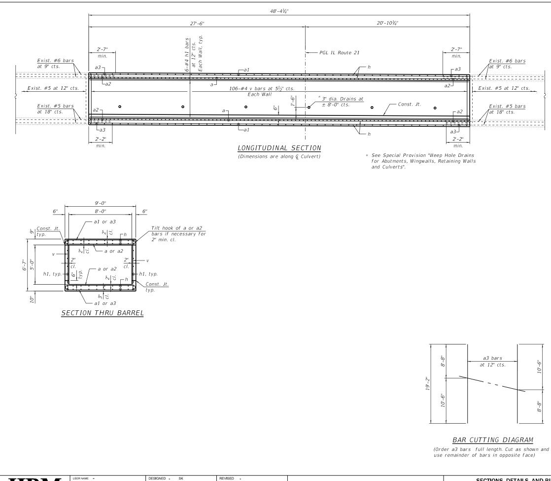
SECTIONS, DETAILS, AND STATE OF ILLINOIS CHECKED - MI, RTB REVISED -S.N. 049-0599 IL 21 (MILWAU **DEPARTMENT OF TRANSPORTATION** PLOT SCALE = DRAWN - SK REVISED -PLOT DATE = DATE - 01/14/2018 REVISED -SHEET S-08 OF S-0 ENGINEERING GROUP, LLC
