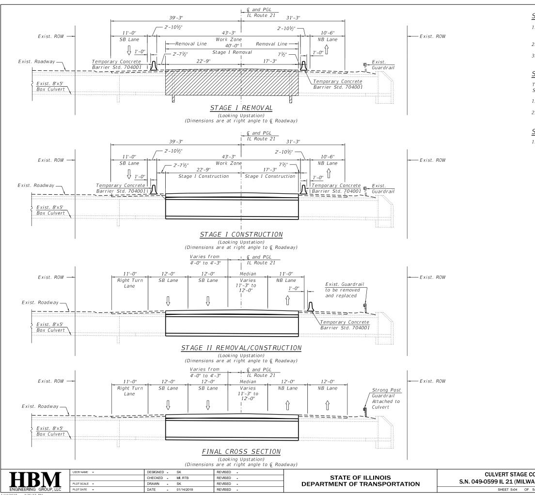
DEL: Default NAME: P<sub>1</sub>/1710-746 IDOT District 1/WO 7 IL21 Culvert Replacement/Sheet/Structural/0490599 S-04 St
