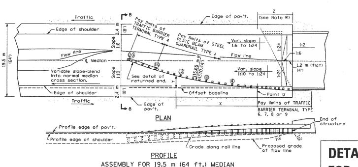
OFFSETS TO FACE OF RAIL DISTANCE m OFFSET m X (ft.) Y (ft.) POST POINT 0 (O) (0)7.60 0.56 4 (24.93)(1.83)1.60 15,14 (8) (5.28)3.16 (10.37) (12) 22.60 (74.16)5.20 (17.05) 29.94 (16) (98,23) 37.13 7.71 20) (121.83) (25.3) 10.70 (24) (144.83)(35.09)
