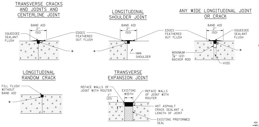
\* HOT ASPHALT CRACK SEALANT
