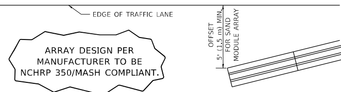
DETAIL "A" IMPACT ATTENUATOR, TEMPORARY (SEE NOTE 5)
