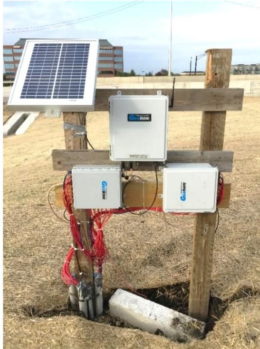
The Contractor shall assist the researchers in the installation of a lightning protection system (rods inserted/embedded in the ground, supplied by researchers) to the data collection locations. The data collection location is where the data acquisition equipment is installed. See photo below.
