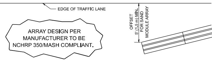
DETAIL "A" IMPACT ATTENUATOR, TEMPORARY (SEE NOTE 5)
