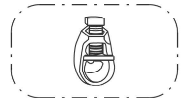
3/4" HEAVY-DUTY GROUND ROD CLAMP BRONZE OR COPPER, UL APPROVED (BURNDY TYPE GRC OR APPROVED EQUAL)
