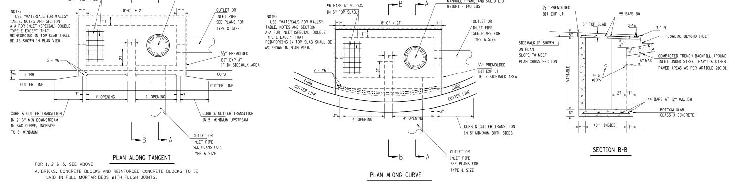
5. WHEN CONSTRUCTED OF MONOLITHIC CONCRETE, USE #4 REINFORCING BARS SPACED AT 12" CENTERS BOTH WAYS IN FLOOR SLAB AND WALLS.
