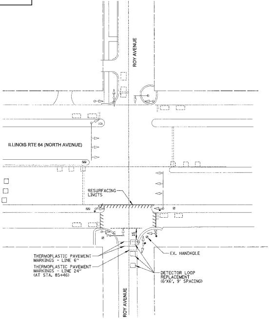
THIS PLAN IS FOR THE SOLE PURPOSE OF DETECTOR LOOP REPLACEMENT
