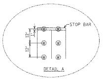
(W) IN PAVEMENT WIRELESS MAGNETOMETER VEHICLE DETECTORS, SENSYS VSN240-T OR APPROVED EQUAL. ALL WIRELESS MAGNETOMETER VEHICLE DETECTORS ARE TO BE PLACED IN A 4" DIA, BY 2.5" DEEP CORE.
