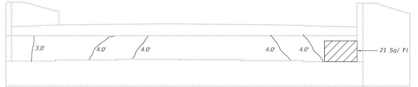
EAST ABUTMENT ELEVATION (SN 098-0062 WB, Looking East)
