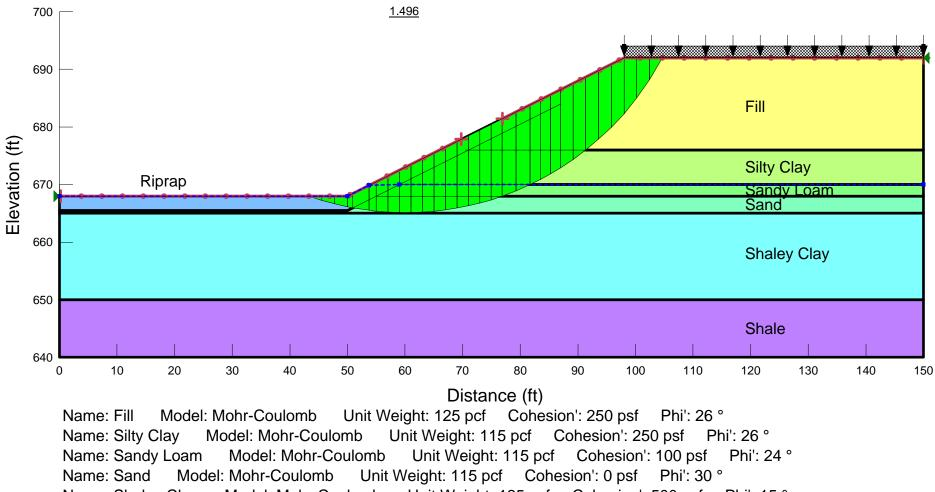
Name: Shaley Clay Model: Mohr-Coulomb Unit Weight: 125 pcf Cohesion': 500 psf Phi': 15 ° Name: Rip Rap Model: Mohr-Coulomb Unit Weight: 135 pcf Cohesion': 0 psf Phi': 38 ° Name: Shale Model: Bedrock (Impenetrable)
