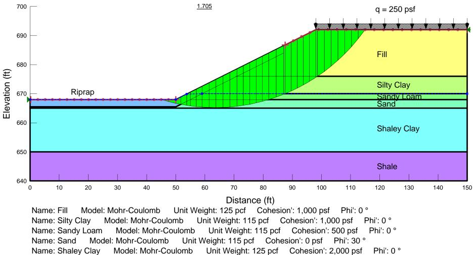
Name: Rip Rap Model: Mohr-Coulomb Unit Weight: 135 pcf Cohesion': 0 psf Phi': 38 ° Name: Shale Model: Bedrock (Impenetrable)
