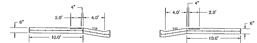
A HIGH SCHOOL PC CONCRETE SIDEWALK PROFILE VIEW C-2 SCALE: NO SCALE
