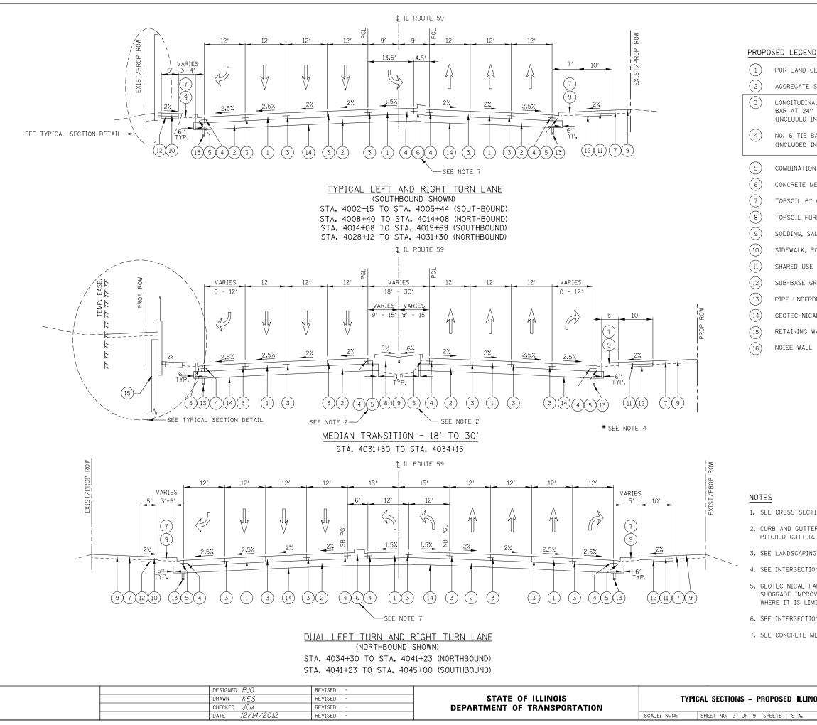
PORTLAND CEMENT CONCRETE PAVEMENT, 10 1/4" (JOINTED)
