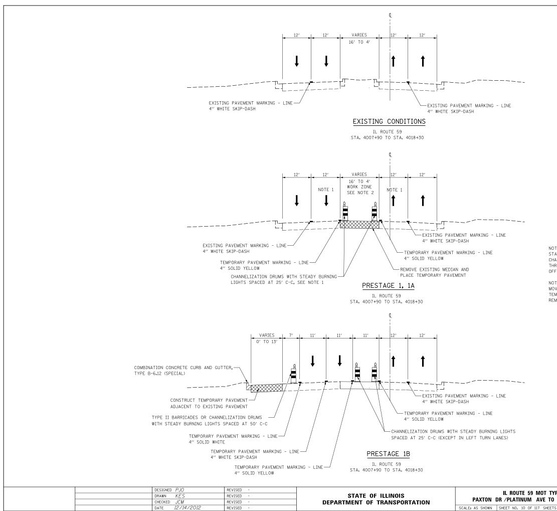
NOTE 1: THE LEFT THROUGH LANE TO BE CLOSED IN ACCORDANCE WITH IDOT STANDARD 701601 DURING CONSTRUCTION WITHIN THE EXISTING MEDIAN. CHANNELIZATION DRUMS SHALL BE RELOCATED ALONG THE ADJACENT THROUGH LANE OPEN TO TRAFFIC. THIS WORK MUST BE DONE DURING OFF-PEAK PERIODS AS DETERMINED BY THE ENGINEER.
