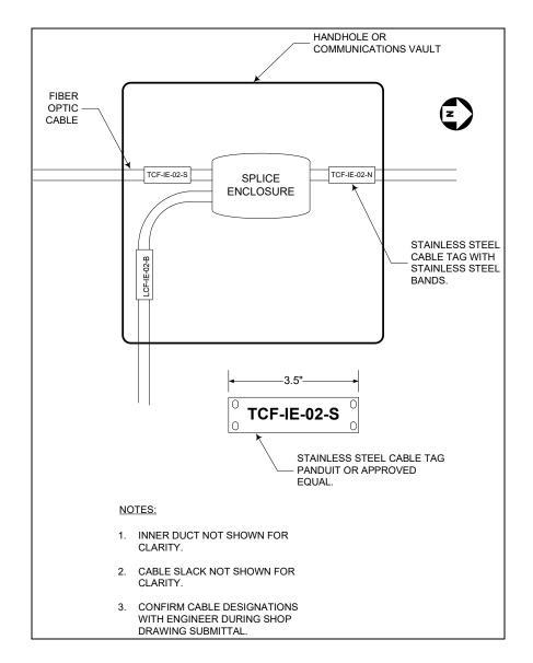
Label the destination of each trunk cable onto the cable in each handhole, vault or cable termination panel.
