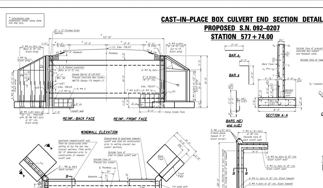
Double Barrel 12'x10'x52' Precast concrete box culvert (M273) Design fill height < 2'
