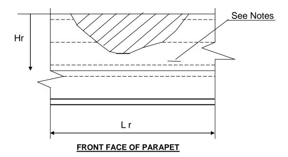
Hr and Lr indicate dimensions for concrete removal. Perimeters of concrete removal areas shall be saw cut 3/4" prior to removal of concrete.
