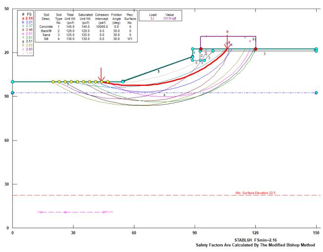
The results of the global stability analysis indicate calculated factors of safety meet or exceed the recommended minimums for each loading case. Below is a summary of the results of the global wall stability analysis.
