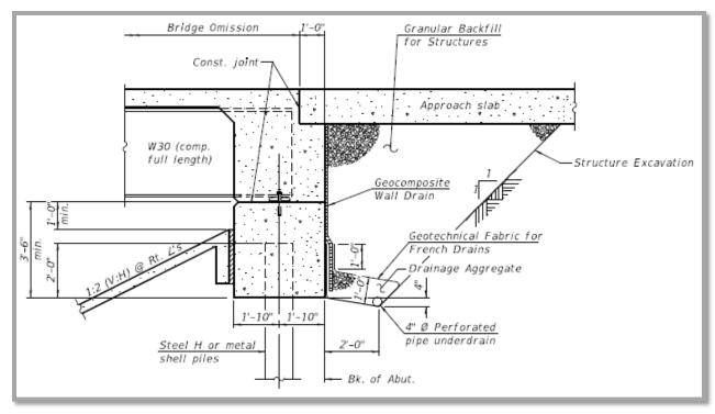
Exhibit 1) Cross-section through integral abutment
