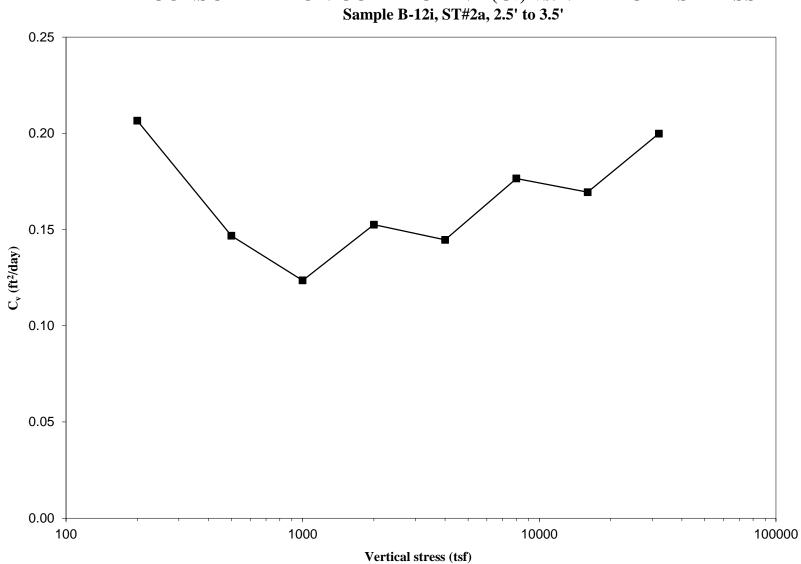
CONSOLIDATION COEFFICIENT (Cv) vs. VERTICAL STRESS
