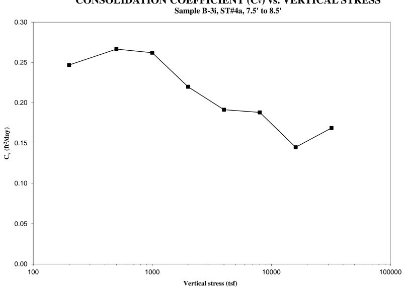
CONSOLIDATION COEFFICIENT (Cv) vs. VERTICAL STRESS
