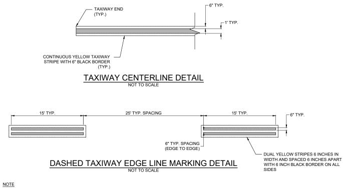
FOR CASES WHERE A TAXIWAY EDGE MARKING INTERSECTS A HOLDING POSITION MARKING THE TAXIWAY EDGE MARKING SHOULD ABUT THE BLACK BORDER, I.E., MAINTAIN A 6-INCH GAP.
