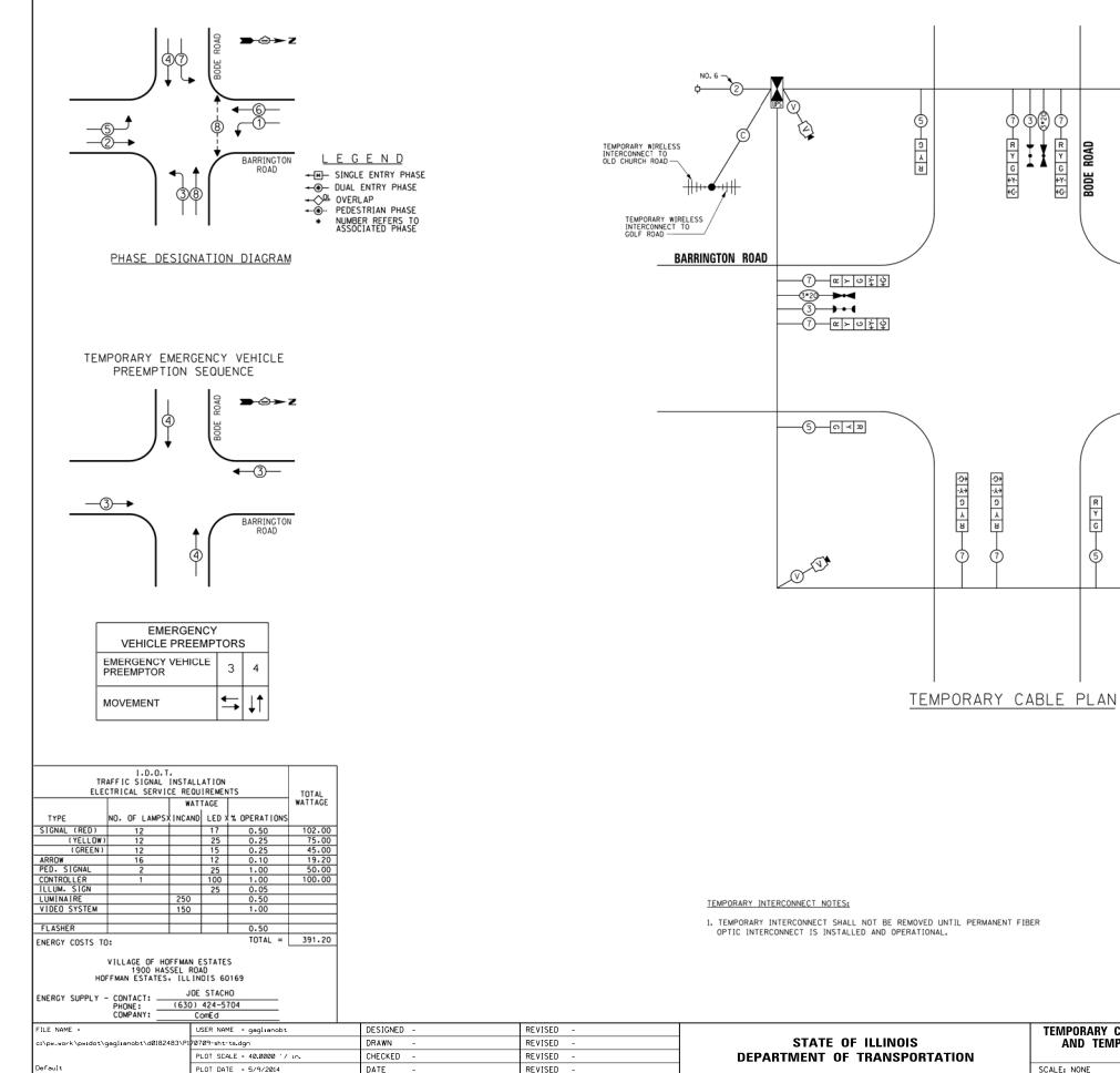
TEMPORARY CABLE PLAN, TEMPORARY AND TEMPORARY EMERGENCY VEH BARRINGTON ROAD SCALE: NONE SHEET OF SHEET
