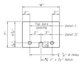
STEEL RETAINER P 1" x 7" x "W" \* Required only with Detail II
