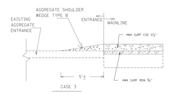
TREATMENT FOR EARTH OR AGGREGATE ENTRANCES AND DRIVEWAYS WITHOUT MAINLINE COMB. CONC. CURB & GUTTER
