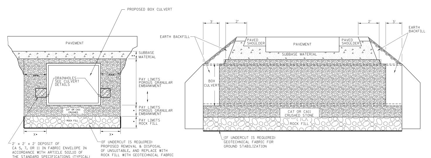
\* IN UNDERCUT AREAS, X = 5 FEET AND ROCK FILL DEPTH SHALL BE 4.5 FEET. IF THERE IS NO UNDERCUT, X = 2 FEET. SEE NOTE 3 THIS SHEET.
