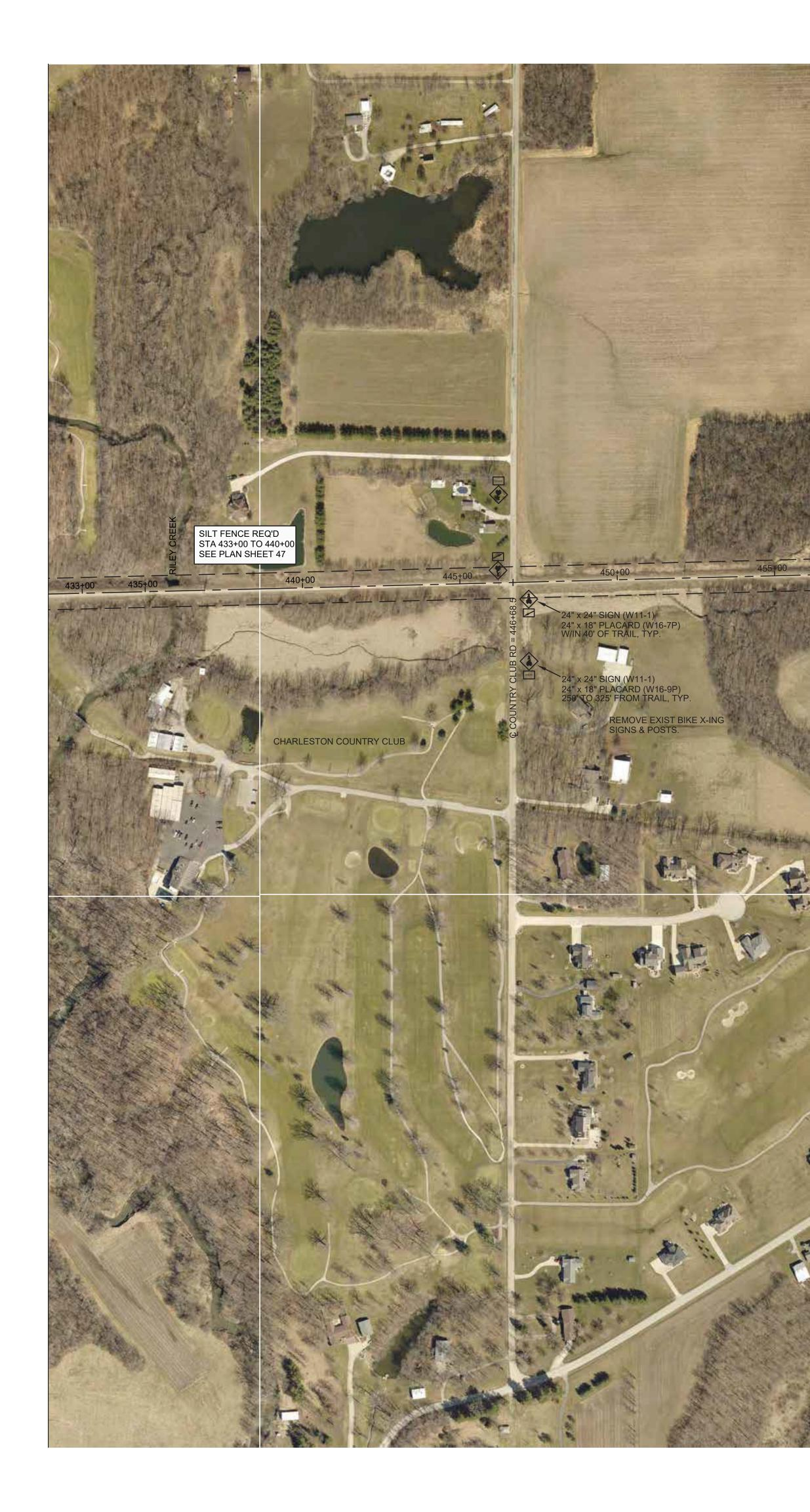
REMOVAL & PROPOSED CONSTRUCTION SCHEDULE COUNTRY CLUB ROAD TO OLD STATE ROAD GROSS LENGTH = 3,578' = 0.68 MILES. PREPARATION OF BASE = 4,650 SQYD HMA SURF CSE, MIX 'C', N70 = 456 TONS GRADING AND SHAPING SHOULDERS = 71 UNITS SEEDING BY OTHERS. SEE SHEET 32 FOR INTERSECTION DETAILS.
